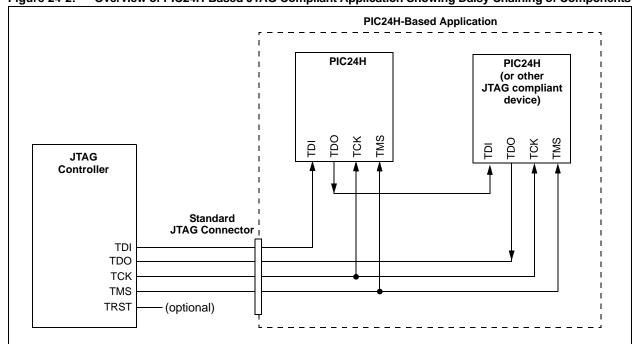
Figure 24-2: Overview of PIC24H-Based JTAG Compliant Application Showing Daisy Chaining of Components
