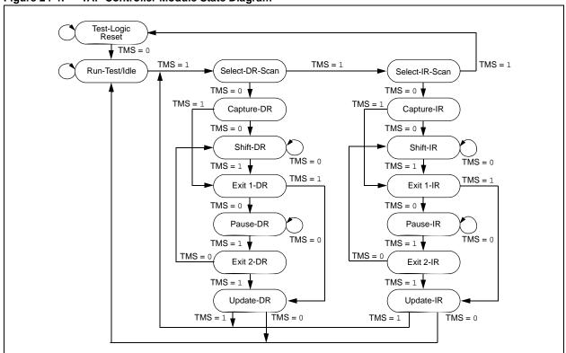
Figure 24-4: TAP Controller Module State Diagram
